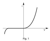
An application of the voltage current curve is given by  $I = I_S \left( exp \frac{V}{V_T} - 1 \right)$ where
